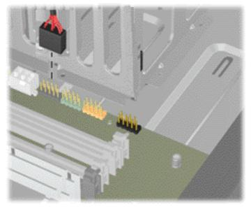
Figure 5-18 Disconnecting the Media Card Reader USB Cable
